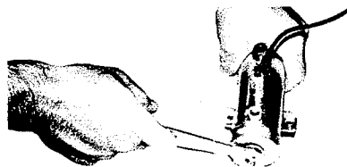
FIGURE 7-4 ELECTRIC FUEL PUMP DISASSEMBLY
