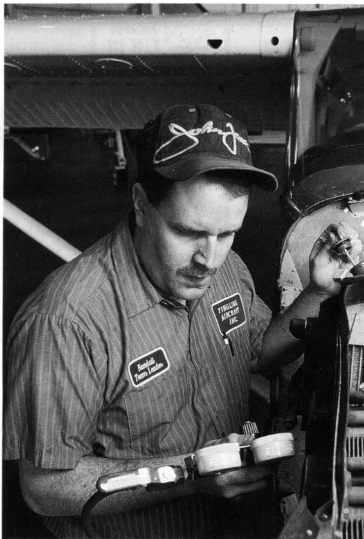
Using a differential compression tester, your mechanic determines how well the engine's cylinders are able to seal in combustion pressure.
